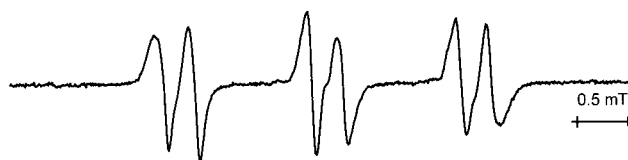
Figure 7. ESR spectrum obtained after thermolysis of ozonized PIB at 100\text{ }^\circ\text{C} in the presence of the radical trap, PBN.
